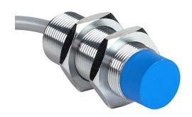
Contrinex inductive proximity sensor, tubular, 18mm diameter x 51mm body, chrome-plated brass housing, PNP, N.O. output, 20mm sensing distance, non-flush, 500 Hz switching frequency, IP67, pigtail.
