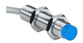
Contrinex inductive proximity sensor, tubular, 12mm diameter x 50mm body, chrome-plated brass housing, PNP, N.O. output, 10mm sensing distance, non-flush, 400 Hz switching frequency, IP67, pigtail.
