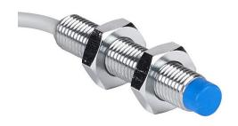
Contrinex inductive proximity sensor, tubular, 8mm diameter x 45mm body, chrome-plated brass housing, NPN, N.O. output, 6mm sensing distance, non-flush, 500 Hz switching frequency, IP67, pigtail.
