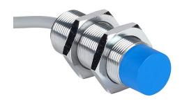
Contrinex inductive proximity sensor, tubular, 18mm diameter x 51mm body, chrome-plated brass housing, NPN, N.O. output, 20mm sensing distance, non-flush, 500 Hz switching frequency, IP67, pigtail.
