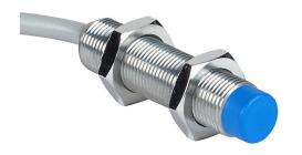
Contrinex inductive proximity sensor, tubular, 12mm diameter x 50mm body, chrome-plated brass housing, NPN, N.O. output, 10mm sensing distance, non-flush, 400 Hz switching frequency, IP67, pigtail.
