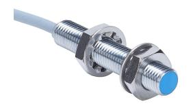
Contrinex inductive proximity sensor, tubular, 8mm diameter x 45mm body, chrome-plated brass housing, 0-5 VDC analog output, 4mm sensing distance, semi-flush, IP67, pigtail.
