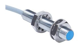
Contrinex inductive proximity sensor, tubular, 8mm diameter x 45mm body, chrome-plated brass housing, 0-5 VDC analog output, 4mm sensing distance, semi-flush, IP67, pigtail.
