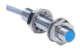
Contrinex inductive proximity sensor, tubular, 8mm diameter x 45mm body, chrome-plated brass housing, 0-10 VDC analog output, 4mm sensing distance, semi-flush, IP67, pigtail.
