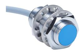
Contrinex inductive proximity sensor, tubular, 18mm diameter x 36mm body, chrome-plated brass housing, 0-10 VDC or 4-20 mA analog output, 10mm sensing distance, semi-flush, IP67, pigtail.
