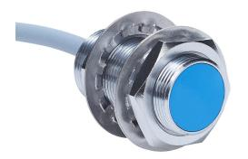
Contrinex inductive proximity sensor, tubular, 18mm diameter x 36mm body, chrome-plated brass housing, 0-5 VDC or 1-5 mA analog output, 10mm sensing distance, semi-flush, IP67, pigtail.
