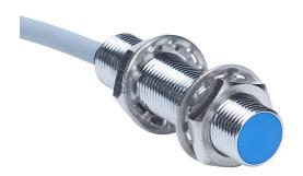
Contrinex inductive proximity sensor, tubular, 12mm diameter x 50mm body, chrome-plated brass housing, 0-5 VDC or 1-5 mA analog output, 6mm sensing distance, semi-flush, IP67, pigtail.
