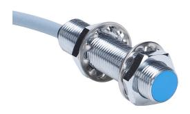
Contrinex inductive proximity sensor, tubular, 12mm diameter x 50mm body, chrome-plated brass housing, 0-10 VDC or 4-20 mA analog output, 6mm sensing distance, semi-flush, IP67, pigtail.
