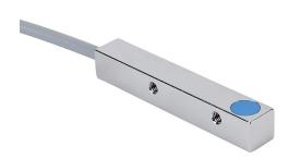
Contrinex inductive proximity sensor, rectangular, 8 x 8 x 50mm body, chrome-plated brass housing, 0-10 VDC analog output, 4mm sensing distance, semi-flush, IP67, pigtail.
