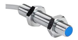
Contrinex inductive proximity sensor, tubular, 8mm diameter x 45mm body, chrome-plated nickel silver housing, PNP, N.C. output, 3mm sensing distance, semi-flush, 1 kHz switching frequency, IP67, pigtail.
