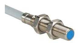
Contrinex inductive proximity sensor, tubular, 5mm diameter x 25mm body, nickel silver housing, PNP, N.C. output, 2.5mm sensing distance, semi-flush, 800 Hz switching frequency, IP67, pigtail.
