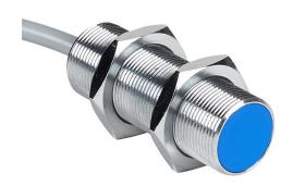
Contrinex inductive proximity sensor, tubular, 18mm diameter x 51mm body, chrome-plated brass housing, PNP, N.C. output, 12mm sensing distance, semi-flush, 600 Hz switching frequency, IP67, pigtail.
