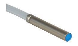
Contrinex inductive proximity sensor, tubular, 4mm diameter x 25mm body, nickel silver housing, PNP, N.C. output, 2.5mm sensing distance, semi-flush, 800 Hz switching frequency, IP67, pigtail.
