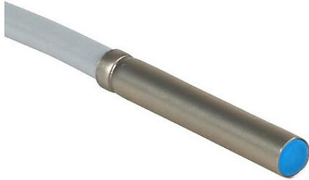
Contrinex inductive proximity sensor, tubular, 4mm diameter x 25mm body, nickel silver housing, PNP, N.C. output, 2.5mm sensing distance, semi-flush, 800 Hz switching frequency, IP67, pigtail.
