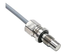
Contrinex inductive proximity sensor, tubular, 8mm diameter x 30mm body, 304 stainless steel housing, PNP, N.O., 1.5mm sensing distance, flush, 800 Hz switching frequency, IP68, pigtail.
