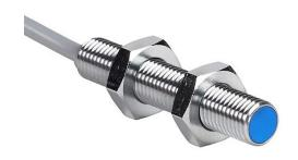
Contrinex inductive proximity sensor, tubular, 8mm diameter x 45mm body, chrome-plated nickel silver housing, PNP, N.O. output, 3mm sensing distance, semi-flush, 1 kHz switching frequency, IP67, pigtail.
