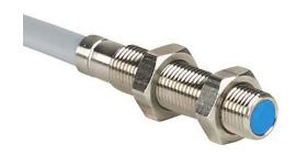
Contrinex inductive proximity sensor, tubular, 5mm diameter x 25mm body, nickel silver housing, PNP, N.O. output, 2.5mm sensing distance, semi-flush, 800 Hz switching frequency, IP67, pigtail.
