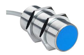
Contrinex inductive proximity sensor, tubular, 30mm diameter x 60mm body, chrome-plated brass housing, PNP, N.O. output, 22mm sensing distance, semi-flush, 200 Hz switching frequency, IP67, pigtail.
