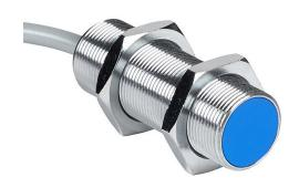
Contrinex inductive proximity sensor, tubular, 18mm diameter x 51mm body, chrome-plated brass housing, PNP, N.O. output, 12mm sensing distance, semi-flush, 600 Hz switching frequency, IP67, pigtail.
