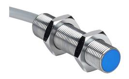
Contrinex inductive proximity sensor, tubular, 12mm diameter x 50mm body, chrome-plated brass housing, PNP, N.O. output, 6mm sensing distance, semi-flush, 800 Hz switching frequency, IP67, pigtail.
