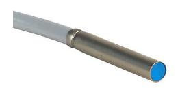
Contrinex inductive proximity sensor, tubular, 4mm diameter x 25mm body, nickel silver housing, PNP, N.O. output, 2.5mm sensing distance, semi-flush, 800 Hz switching frequency, IP67, pigtail.
