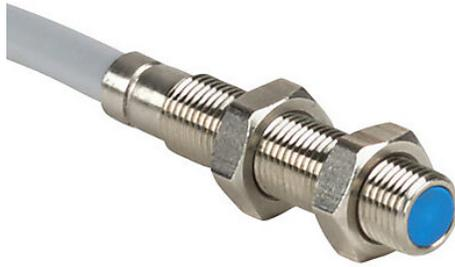
Contrinex inductive proximity sensor, tubular, 5mm diameter x 25mm body, nickel silver housing, NPN, N.C. output, 2.5mm sensing distance, semi-flush, 800 Hz switching frequency, IP67, pigtail.
