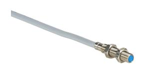
Contrinex inductive proximity sensor, tubular, 5mm diameter x 25mm body, nickel silver housing, NPN, N.O. output, 2.5mm sensing distance, semi-flush, 800 Hz switching frequency, IP67, pigtail.
