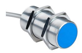
Contrinex inductive proximity sensor, tubular, 30mm diameter x 60mm body, chrome-plated brass housing, NPN, N.O. output, 22mm sensing distance, semi-flush, 200 Hz switching frequency, IP67, pigtail.
