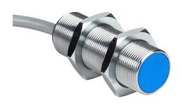
Contrinex inductive proximity sensor, tubular, 18mm diameter x 51mm body, chrome-plated brass housing, NPN, N.O. output, 12mm sensing distance, semi-flush, 600 Hz switching frequency, IP67, pigtail.
