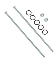
NITRA mounting kit, for use with 6-station DVP-2C or DVP-3C series valves, includes (2) #8-32 x 6in screws, (2) #8 lock nuts and (5) Viton O-rings.
