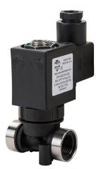
NITRA solenoid valve, 3-way, 2-position, N.C., glass-filled nylon body, 3/8in female NPT inlet(s), 3/8in female NPT outlet(s), Cv=0.315, 24 VDC operating voltage, 18mm DIN style wiring plug.
