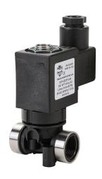
NITRA solenoid valve, 3-way, 2-position, N.C., glass-filled nylon body, 3/8in female NPT inlet(s), 3/8in female NPT outlet(s), Cv=0.315, 24 VAC operating voltage, 18mm DIN style wiring plug.
