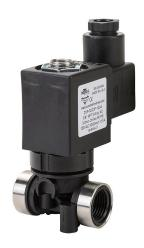
NITRA solenoid valve, 3-way, 2-position, N.C., glass-filled nylon body, 3/8in female NPT inlet(s), 3/8in female NPT outlet(s), Cv=0.315, 120 VAC operating voltage, 18mm DIN style wiring plug.
