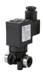
NITRA solenoid valve, 3-way, 2-position, N.C., glass-filled nylon body, 1/4in female NPT inlet(s), 1/4in female NPT outlet(s), Cv=0.245, 24 VDC operating voltage, 18mm DIN style wiring plug.
