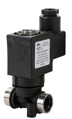
NITRA solenoid valve, 3-way, 2-position, N.C., glass-filled nylon body, 1/4in female NPT inlet(s), 1/4in female NPT outlet(s), Cv=0.245, 24 VAC operating voltage, 18mm DIN style wiring plug.
