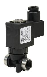
NITRA solenoid valve, 3-way, 2-position, N.C., glass-filled nylon body, 1/4in female NPT inlet(s), 1/4in female NPT outlet(s), Cv=0.245, 120 VAC operating voltage, 18mm DIN style wiring plug.
