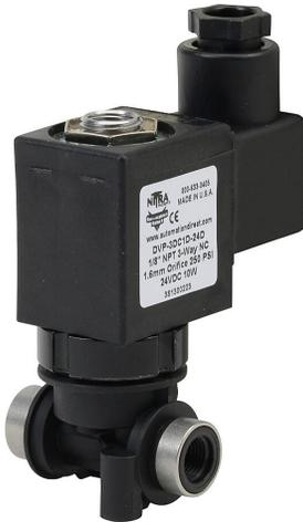
NITRA solenoid valve, 3-way, 2-position, N.C., glass-filled nylon body, 1/8in female NPT inlet(s), 1/8in female NPT outlet(s), Cv=0.12, 24 VDC operating voltage, 18mm DIN style wiring plug.
