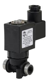
NITRA solenoid valve, 3-way, 2-position, N.C., glass-filled nylon body, 1/8in female NPT inlet(s), 1/8in female NPT outlet(s), Cv=0.12, 24 VDC operating voltage, 18mm DIN style wiring plug.
