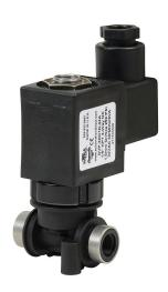
NITRA solenoid valve, 3-way, 2-position, N.C., glass-filled nylon body, 1/8in female NPT inlet(s), 1/8in female NPT outlet(s), Cv=0.12, 24 VAC operating voltage, 18mm DIN style wiring plug.
