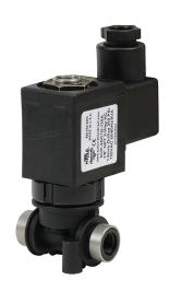
NITRA solenoid valve, 3-way, 2-position, N.C., glass-filled nylon body, 1/8in female NPT inlet(s), 1/8in female NPT outlet(s), Cv=0.12, 120 VAC operating voltage, 18mm DIN style wiring plug.
