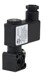
NITRA solenoid valve, 3-way, 2-position, N.C., glass-filled nylon body, 1/8in female NPT inlet(s), 1/8in female NPT outlet(s), stackable, Cv=0.08, 24 VDC operating voltage, 11mm DIN style wiring plug.
