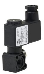
NITRA solenoid valve, 3-way, 2-position, N.C., glass-filled nylon body, 1/8in female NPT inlet(s), 1/8in female NPT outlet(s), stackable, Cv=0.08, 24 VAC operating voltage, 11mm DIN style wiring plug.
