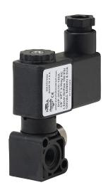
NITRA solenoid valve, 3-way, 2-position, N.C., glass-filled nylon body, 1/8in female NPT inlet(s), 1/8in female NPT outlet(s), stackable, Cv=0.08, 120 VAC operating voltage, 11mm DIN style wiring plug.
