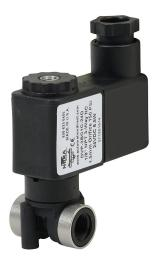
NITRA solenoid valve, 3-way, 2-position, N.C., glass-filled nylon body, 1/8in female NPT inlet(s), 1/8in female NPT outlet(s), Cv=0.08, 24 VDC operating voltage, 11mm DIN style wiring plug.
