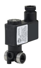
NITRA solenoid valve, 3-way, 2-position, N.C., glass-filled nylon body, 1/8in female NPT inlet(s), 1/8in female NPT outlet(s), Cv=0.08, 24 VAC operating voltage, 11mm DIN style wiring plug.
