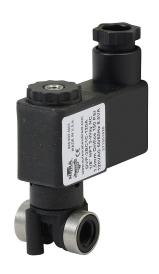
NITRA solenoid valve, 3-way, 2-position, N.C., glass-filled nylon body, 1/8in female NPT inlet(s), 1/8in female NPT outlet(s), Cv=0.08, 120 VAC operating voltage, 11mm DIN style wiring plug.
