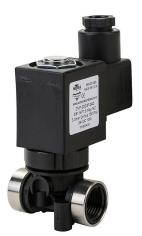
NITRA solenoid valve, 2-way, 2-position, N.C., glass-filled nylon body, 3/8in female NPT inlet(s), 3/8in female NPT outlet(s), Cv=0.315, 24 VDC operating voltage, 18mm DIN style wiring plug.
