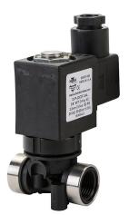
NITRA solenoid valve, 2-way, 2-position, N.C., glass-filled nylon body, 3/8in female NPT inlet(s), 3/8in female NPT outlet(s), Cv=0.315, 24 VAC operating voltage, 18mm DIN style wiring plug.
