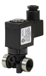
NITRA solenoid valve, 2-way, 2-position, N.C., glass-filled nylon body, 3/8in female NPT inlet(s), 3/8in female NPT outlet(s), Cv=0.315, 120 VAC operating voltage, 18mm DIN style wiring plug.
