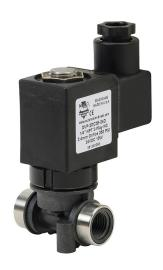
NITRA solenoid valve, 2-way, 2-position, N.C., glass-filled nylon body, 1/4in female NPT inlet(s), 1/4in female NPT outlet(s), Cv=0.245, 24 VDC operating voltage, 18mm DIN style wiring plug.
