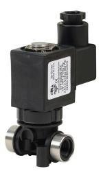
NITRA solenoid valve, 2-way, 2-position, N.C., glass-filled nylon body, 1/4in female NPT inlet(s), 1/4in female NPT outlet(s), Cv=0.245, 24 VAC operating voltage, 18mm DIN style wiring plug.
