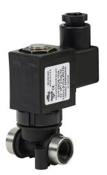
NITRA solenoid valve, 2-way, 2-position, N.C., glass-filled nylon body, 1/4in female NPT inlet(s), 1/4in female NPT outlet(s), Cv=0.245, 120 VAC operating voltage, 18mm DIN style wiring plug.
