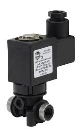
NITRA solenoid valve, 2-way, 2-position, N.C., glass-filled nylon body, 1/8in female NPT inlet(s), 1/8in female NPT outlet(s), Cv=0.12, 24 VDC operating voltage, 18mm DIN style wiring plug.
